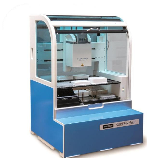
The SURFE<sup>2</sup>R (surface electrogenic event reader) technology allows the investigation of electrogenic transporters (symporters, exchangers and uniporters) and pumps.
